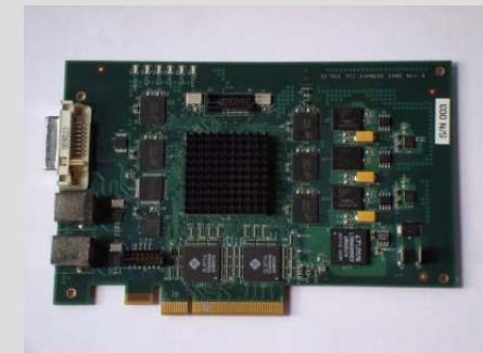
Segue II board for real-time 3D LIDAR shape matching & 3D/4D model building
